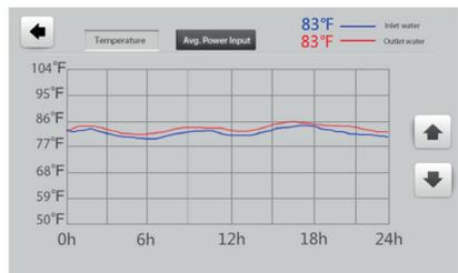
The temperature curve automatically updates every hour, and the curve record can be stored for 60 days
