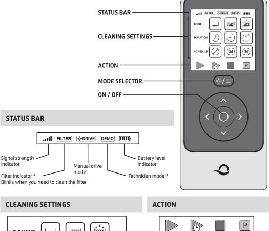
CLEANING //// MODE Floor only Floor, walls and Ultra clean Start later Stop Pick me up Start waterline Start Starts cleaning immediately, according to DURATION selected settings. Start later Starts cleaning after 1 hour. Short cycle Long cycle Default cycle Stop Stops the robot in its place and turns it off. (2d SCHEDULE ( 3d ) Pick me up \* Ρ The robot will come to the surface of the pool, for easy pickup. Clean every Schedule disabled Clean every 2nd day 3rd day \* For specific models only
